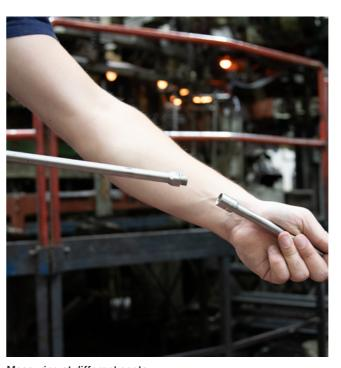
Measuring at different spots It's up to you: Simply extend the probe from 1 meter to 2 meters if necessary. At both lengths it can be equipped with a thermo couple
