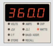
All keyboard entries appear on this display for inspection before they are actioned by pressing the "confirm" key.
