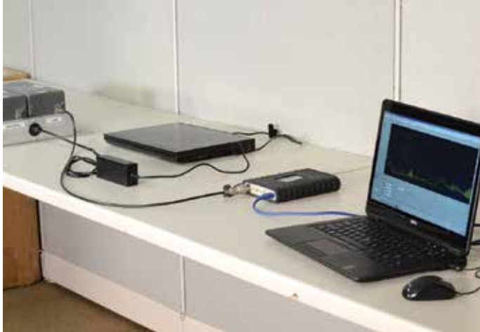
Figure 13. Basic pre-compliance conducted emissions test setup.
