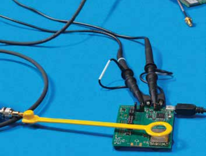
Figure 16. A near field probe can be used to discover the location of unintended RF emissions.
