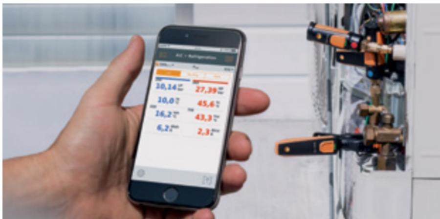
With the AC/R kit, you can measure high-side and low-side pressures and temperatures of A/C and refrigeration systems
