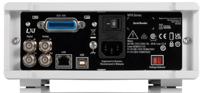
Rear panel of R&S®NPA instruments
