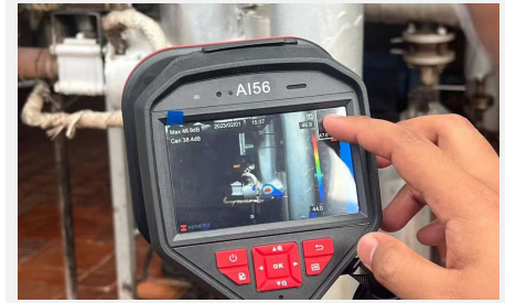
Gas Leakage Detection
