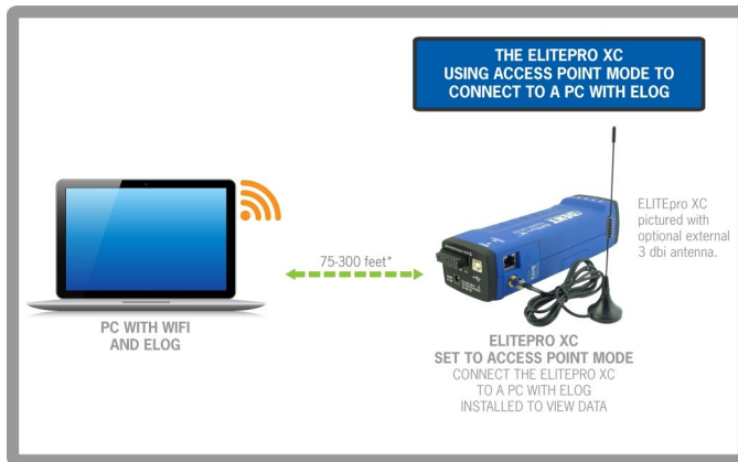
Access Point Mode using ELOG to interface with an ELITEpro XC with Wi-Fi.
