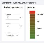
Description: This is likely to be a very strong <u>sufface or internal discharge</u>. Surface or internal discharges on cables, terminations, and joints will progress over time and might rapidly escalate to insulation breakdown. Recommendation: Immediate action, Visual inspection. Cleaning of polluted surfaces. Repair or replacement of
