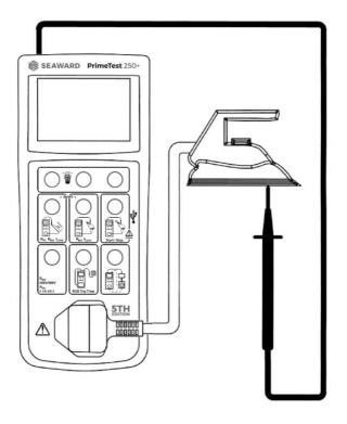
Figure 3. Testing CLI appliances, no mains leakage
