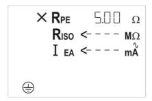
If the measured value is less than the pre-set pass/fail threshold, the measured value is displayed and the unit indicates a pass result, as shown below.
