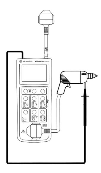
Figure 5. Testing CLI appliances, mains leakage
