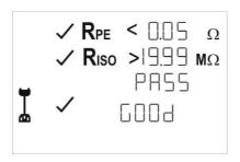
Note: If the tested cord has a wiring fault, one of the following enunciators will be illuminated in place of GOOd
