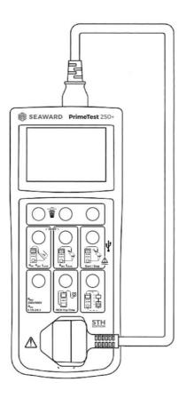
Figure 7. Testing IEC Leads
