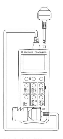
Figure 9. Testing Plug Top RCD
