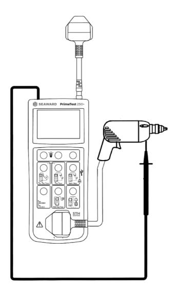
Figure 6. Testing CLII appliances, mains leakage
