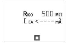
Note: The power switch on the appliance under test must be in the ON position to perform an insulation test. If no appliance is detected the PrimeTest 250+ will display the following.
