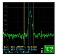
A marker position frequency counter is incorporated for accurate measurement of signal frequencies.
