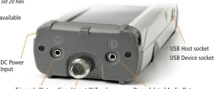
Trigger In/Out Signal Input (N Type) Demodulated Audio Out
