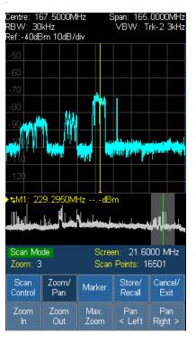
Scan Mode is an entirely different mode of operation in which a narrow RBW can be set resulting in a much higher number of data points being collected - up to 210,000 points.
