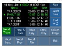
Files are stored under either default file names, or userchosen file names entered from an alpha-numeric keypad.
