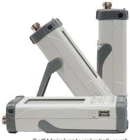
The PSA Series 5 can be used vertically, as well as horizontally or on its tilt stand.
