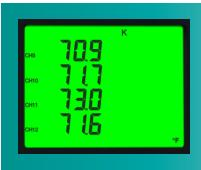
Extech's 12-Channel datalogging thermometer allows for a wide-range of applications with 6 Thermocouple types (J, K, E, T, R,S). It displays CH1 to CH8 or CH9 to CH12 on screen and data can be recorded from all 12 channels simultaneously onto an SD card in Excel® format for further analysis.
