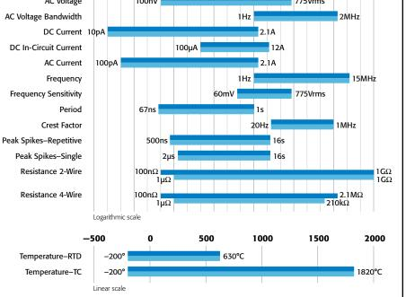
Both the 2001 and 2002 provide exceptional measurement range. In addition, the 2002 offers extended DCV and resistance measurement capabilities.
