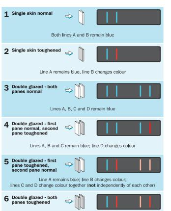
The Merlin Lazer TGi will identify whether or not the glass being tested has been subject to a toughening process. It does not guarantee that glass indicated as being toughend meets BSI standards.
