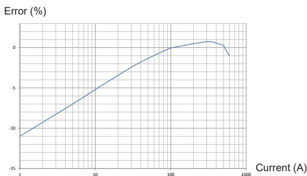
Typical phase error curve at 60Hz
