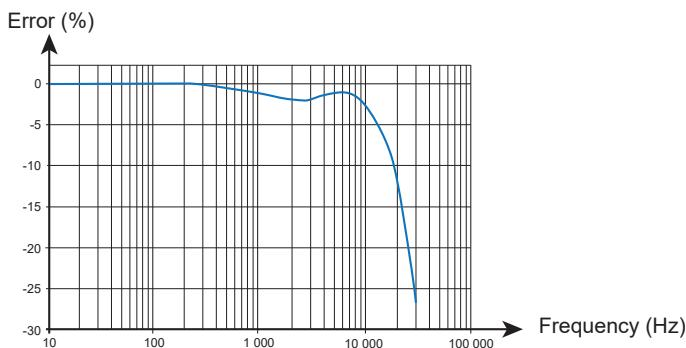
Typical phase versus frequency error curve at 100A
