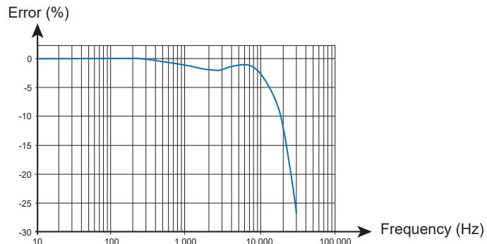
Typical phase error versus frequency curve at 100A
