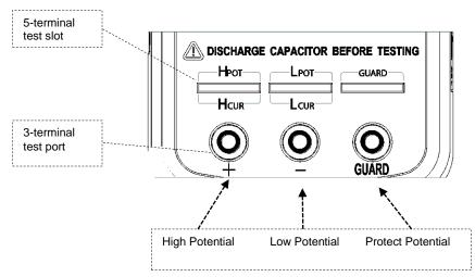
Figure 3 - Test Ports
