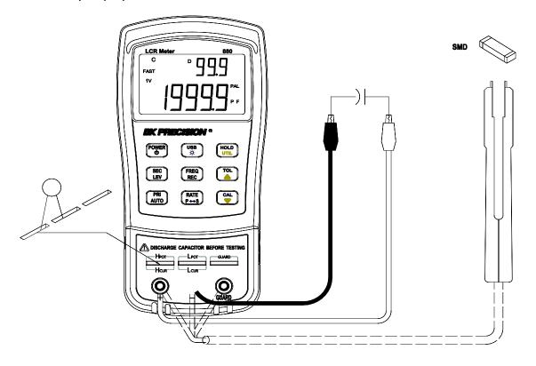
Figure 12 - Capacitance Measurement Setup
