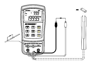
**Figure 9 - Inserting Components to Inputs**
