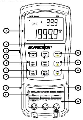
Figure 1 - Front Panel Display
