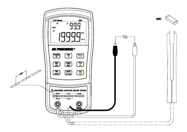
Figure 13 – AC Resistance Measurement Setup
