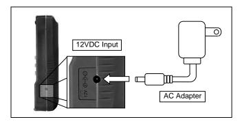
Figure 6 - Connecting AC Adapter to Meter
