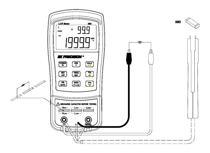
Figure 11 - Inductance Measurement Setup
