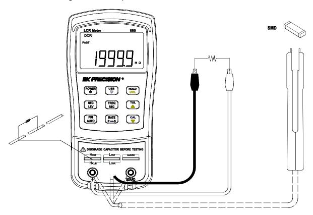
Figure 14 - DCR Measurement Setup
