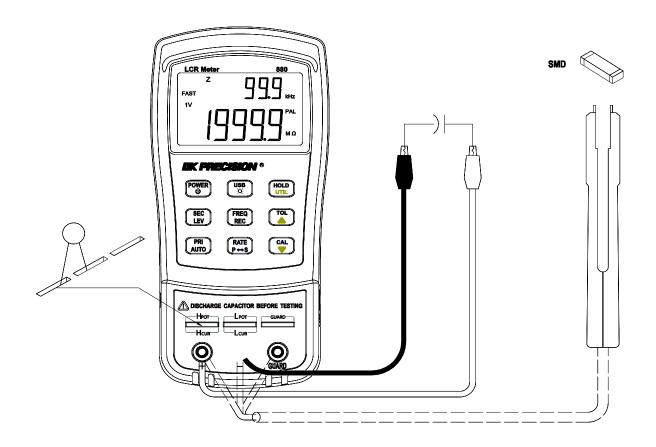
Figure 15 - Impedance Measurement Setup
