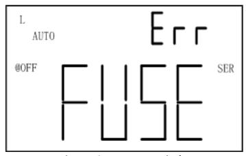
Figure 10 - Fuse Error Display
