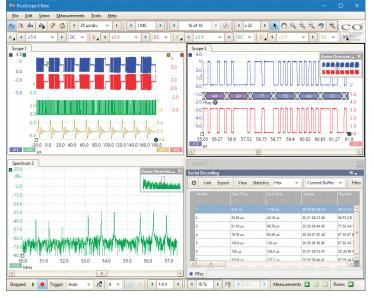
The PicoScope 6 software takes advantage of the display size and resolution and processing power of your PC – in this case displaying four analog signals, a zoomed view of two of the signals (undergoing serial decoding), and a spectrum view of a third, all at the same time. Unlike a conventional benchtop oscilloscope, the size of the display is limited only by the size of your computer monitor. The software is also easy to use on touch-screen devices – you can pinch to zoom and drag to scroll.
