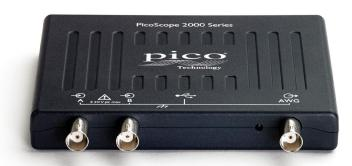
2-channel oscilloscope: 2206B, 2207B and 2208B
