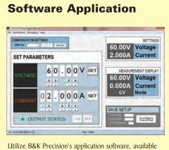
Utilize B&K Precision's application software, available for download at www.bkprecision.com. This software provides a virtual front panel and a simple data logging function to store and log data to a text or CSV file.
