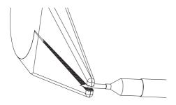
Use pliers to grip and pull the probe carefully out of its contact socket.
