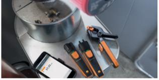
With the Heating kit, you can determine gas flow and static pressure, measure temperature of radiators, and much more
