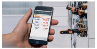
With the AC/R kit, you can measure high-side and low-side pressures and temperatures of A/C and refrigeration systems
